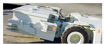
With the ability to engage a battery from below grade, and to vary the ground clearance of the battery in undulating conditions, the versatility of the Bucyrus Scoop is able to thrive in varying mining environments.
