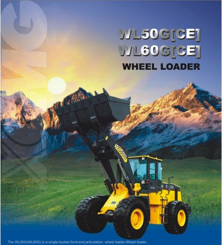
The WL50G(WL60G) is a single-bucket,fornt-end,articulation, wheel loader. Wheel loader. It is adaptive to shovel or transfer such loose material as earth/clay,sand/gravel,aggrgate and rock,and carrying out such tasks as towing,ground leveling,stacking and piling in building site,port,quay,station,yard and so on. So it is a multi-purpose and efficient earth-moving machine.
