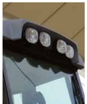
4 front working lights and 4 rear working lights (except B90B: 2 front + 2 rear)
