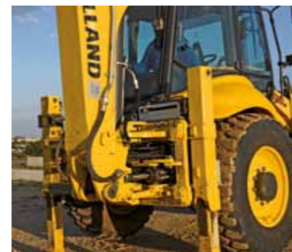
Hydraulic side shift (option): Fast and accurate positioning of the boom without damaging the ground
