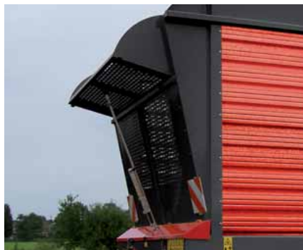
A straight front panel with a manually adjustable front flap. Hydraulic operation is available as option.
