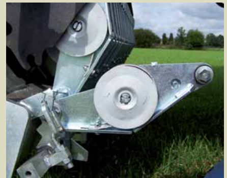
The knives are individually protected against foreign obstacles.
