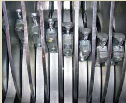
The input tines can be easily changed by releasing the bolt.
