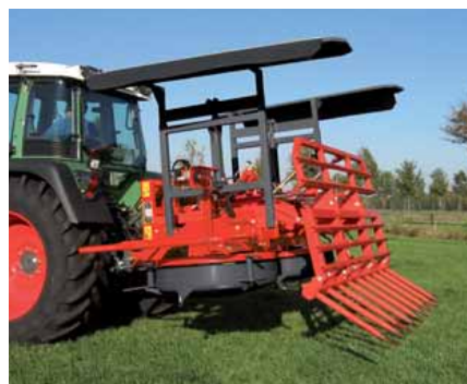
Silodisk VARIO can be fitted with a silo fork.
