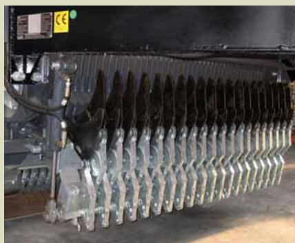
Chop length can be easily set for 38 or 76 mm.
