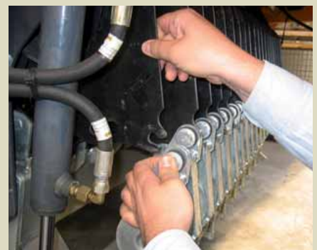
The knives are quickly released and changed.
