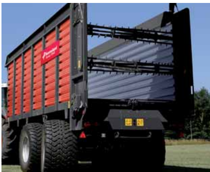
Two distribution rollers available for 12040, 1245 and 12050 for an even more efficient unloading.
