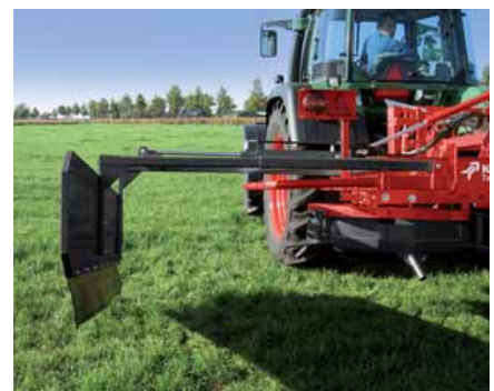
Silodisk VARIO offers hydraulic adjustment of the swath board for working widths up to 6 m.
