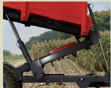
Hydraulically hoisted container using four scissor-action cylinders.
