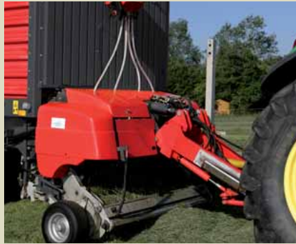
The large 1.85 m pickup with roller crop guard for a smoother material flow.
