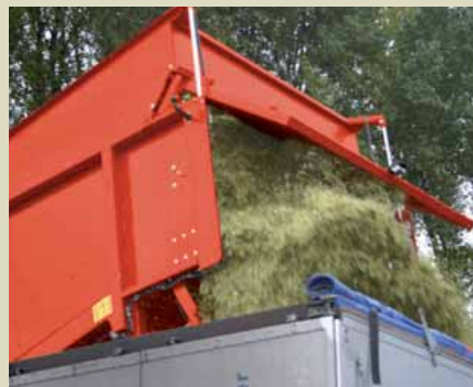
Side and rear walls are pushed upwards during unloading.
