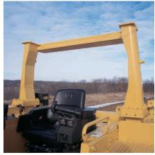
**Optional Roll Over Protective Structure.** Provides for increased operator protection.
