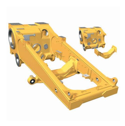
Frame and Castings. Case and frames are built to absorb high impact shock loads and torsional forces. Castings are strategically located within the frame to add additional strength. Caterpillar uses robotic welding techniques in the assembly of the case and frames. This insures quality and reliability throughout the structure. The one-piece all welded chassis provides superior strength over bolted designs, and provides stiffness and durability.
