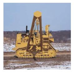
**Roller Frames.** Roller frames are tubular, to resist bending and twisting.
