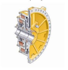
**Steering Clutch and Brakes.** Oil cooled, hydraulically actuated, large diameter plates and clutch discs provide higher torque capacity and increased service life.
