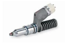
Electronic Unit Injector (EUI). The mechanically actuated, electronically controlled unit injector combines an electronic actuator, pump assembly and nozzle into a single, compact unit for reliability and durability. The 3176C fuel system has been tested in thousands of engines in some of the most demanding applications and environments around the world.
