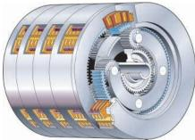
**Transmission.** The proven planetary power shift transmission features three speeds forward and three speeds reverse and utilizes large diameter, high capacity, oil cooled clutches. To maximize the life of the transmission, the planetary design distributes loads and stresses over multiple gears.
