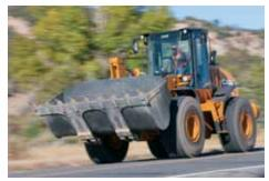
The five-speed transmission with lock-up torque converter option provides faster acceleration, quicker cycle times and higher travel speeds – plus lower fuel consumption
