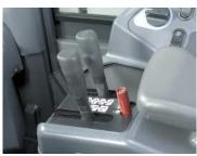
forward or rearward and the large size arm rest can be adjusted up or down to provide the operator with a variety of comfortable operating positions.
