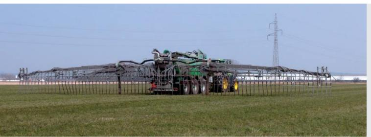
The SAMSON slurry tankers are delivered from 15,000 litres to 25,000 litres. As standard PG is mounted with SAMSON SlurryMaster 6000 dosing computer, and the tanker can be delivered with a large number of accessories and extra equipment.
