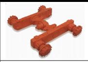
Rear axle is tandem drive. Each tandem assembly oscillates and pivots on a tandem hub bushing. Differential hydraulic lock is operator controlled. Outboard wet disc brakes on each wheel.
