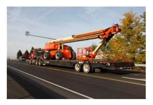
Compact transport dimensions allowing for transport on vehicles capable of carrying 22 ton.
