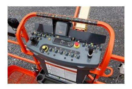
New LCD Display, mounted to the top of JLG standard control panel.
