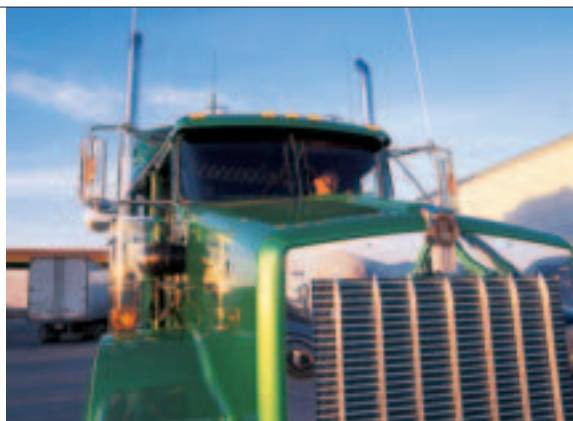
A sloped hood gives the driver a much better view – offering more in-front-of-the-truck visibility than straight hood conventionals.
