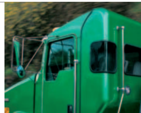
Optional cab corner windows help drivers who need to see better in reverse, at intersections and around the job site.
