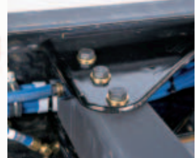
Heavy-duty crossmembers and 3-hole gussets strengthen a T800's backbone, preparing it for the pounding your job dishes out. They can be replaced in less than 10 minutes with no special tools.
