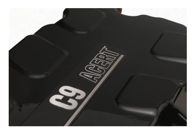
**Engine.** Six-cylinder, turbocharged engine built for power, reliability, and economy will allow the machine to consistently perform at high levels. The Cat® C9 engine is designed for low emissions and will meet EPA Tier 3 emissions requirements.
