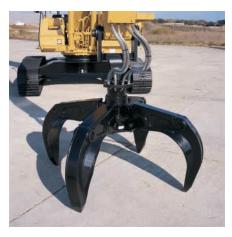
**Orange Peel Grapples.** The 0.96 m<sup>3</sup> (1.25 yd<sup>3</sup>) and the 1.15 m<sup>3</sup> (1.5 yd<sup>3</sup>) Orange Peel Grapples are available attachments.
