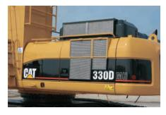
**Cooling System.** External debris filters allow easy access for cleaning. This prevents clogging from dirt and dust entering the cooling system. The optional automatic reversing fan purges dirt and dust from the cooling system.
