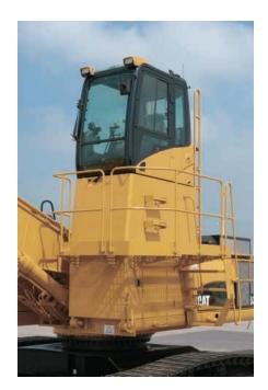
**Fixed Riser.** Cat® designed and built, 1.95 m (6'5") manual tilt cab riser provides for operating height with excellent visibility for loading and unloading processing equipment, trucks, and rail cars. Access to the cab is provided by a ladder to the platform extending around the cab riser. This platform allows for windshield cleaning. The cab riser can be manually tilted forward 90 degrees for shipping.
