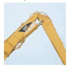
**Dual Stick Cylinders.** Provides excellent geometry for working close in to the machine or at full reach.
