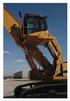
**Hydraulic Cab Riser.** Optional hydraulic cab riser provides up to 2.6 m (8'6") of additional operating height. There is easy access to the cab platform provided by handrails attached to the riser.
