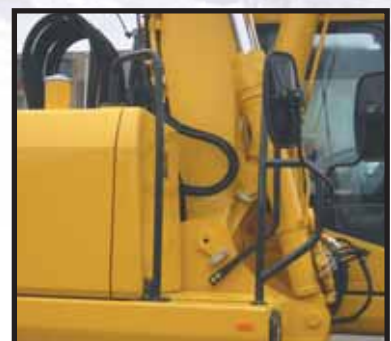
Large handrail for safe access
