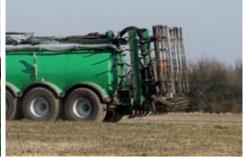
The vertical distributor can be mounted with a hydraulic gate valve, which makes emptying of the stone trap more practical. The gate valve can be used to empty the distributor before transport on the roads.
