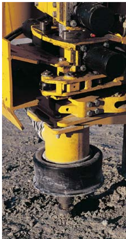
The Atlas Copco double drill tube support with hydraulic breakout table for straighter holes.
