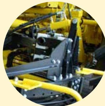
Separate hydraulic height adjustment for flow gate in first turbine
