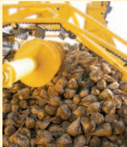
Automatic control for the emptying of the beet tank - with 2 preset delivery heights
