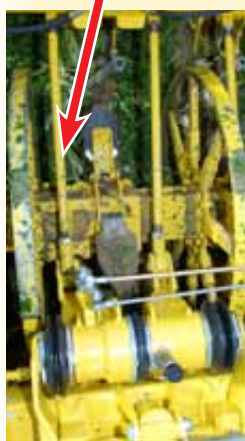
Maintenance-free linear guide
