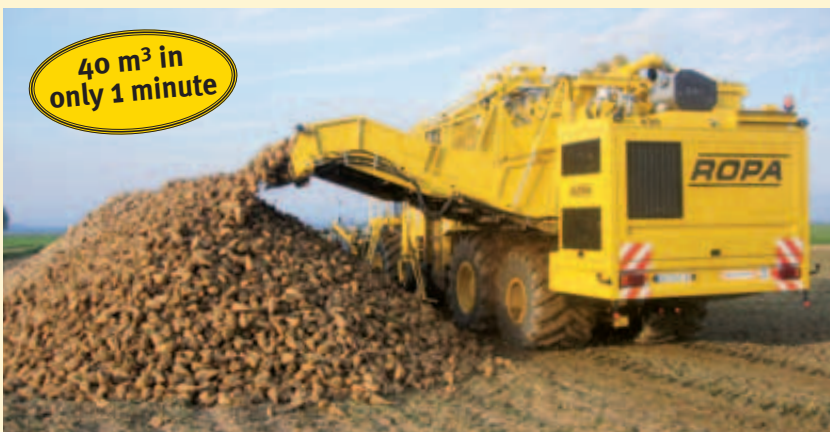
Automatic control for the emptying of the beet tank - with 2 preset delivery heights
