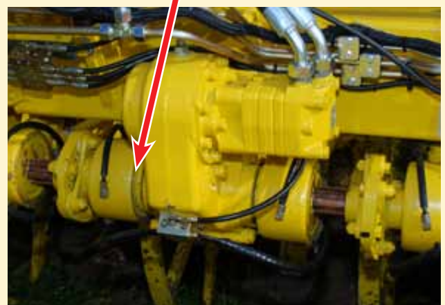
Oscillating share motion with spur gear drive
