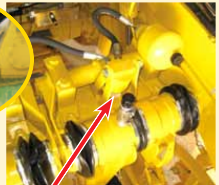
Hydraulic stone protection on top of frame, maintenance-free linear guide
