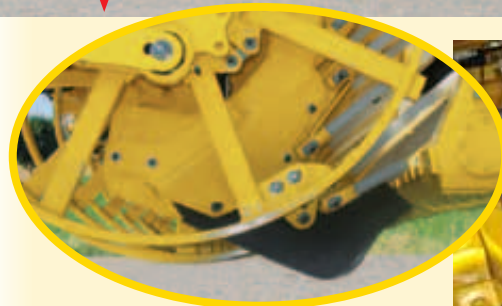
Optimal positioning of the depth sensor wheels to the lifting shares
