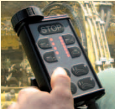
Automatic control for the emptying of the beet tank - with 2 preset delivery heights
