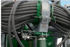
SAMSON drip hose systems can also be equipped with ADS (anti-dripping system), ensuring that the hoses are fully blocked and don't drip during transportation. SB drip hose booms with ADS can be from 12 to 20 m wide.
