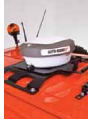
The Auto-Guide 2 TopDock, which houses the GPS antenna, receiver and dynamic measuring, can be easily transferred to any Auto-Guide 2 Ready machine.
