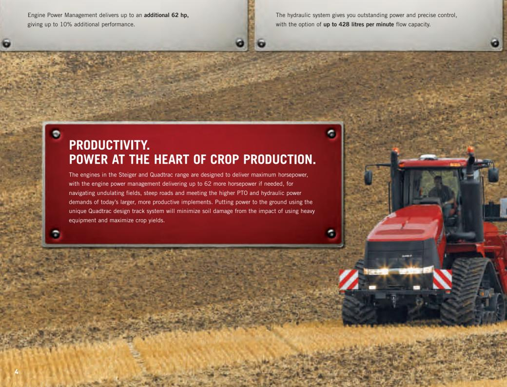
Optimum traction at all times with minimum ground pressure makes Conventional articulated steering gives the Steiger and Quadtrac Series full-power turns within 5.7 m. the Quadtrac the ideal tractor for the heaviest ground conditions.
