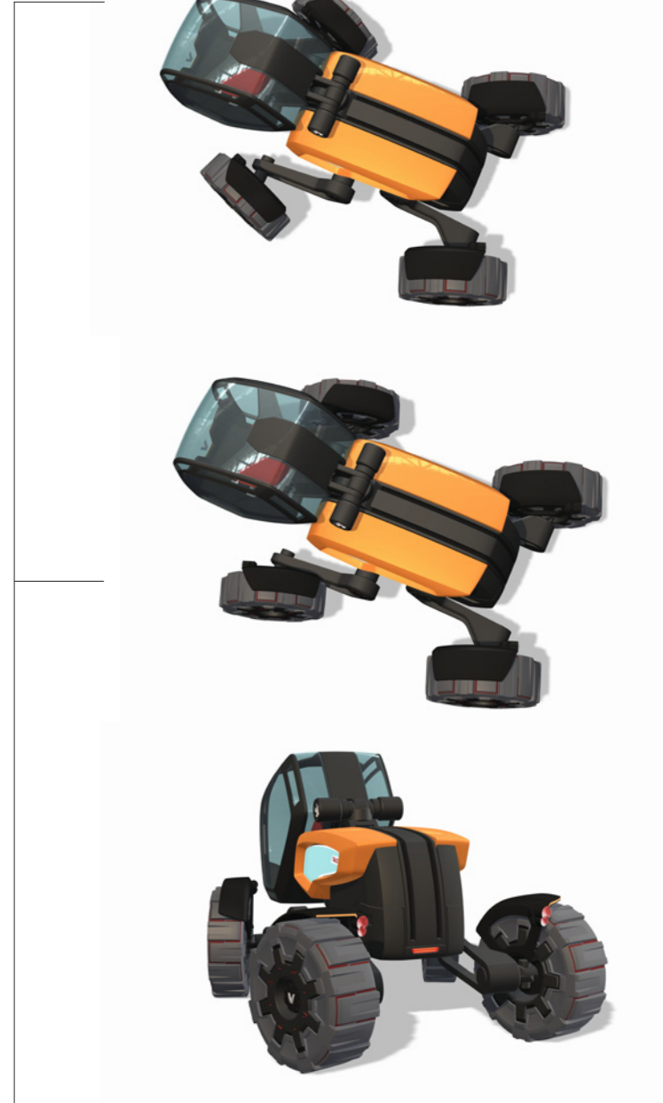
Four wheel steering allows multiple driving modes
