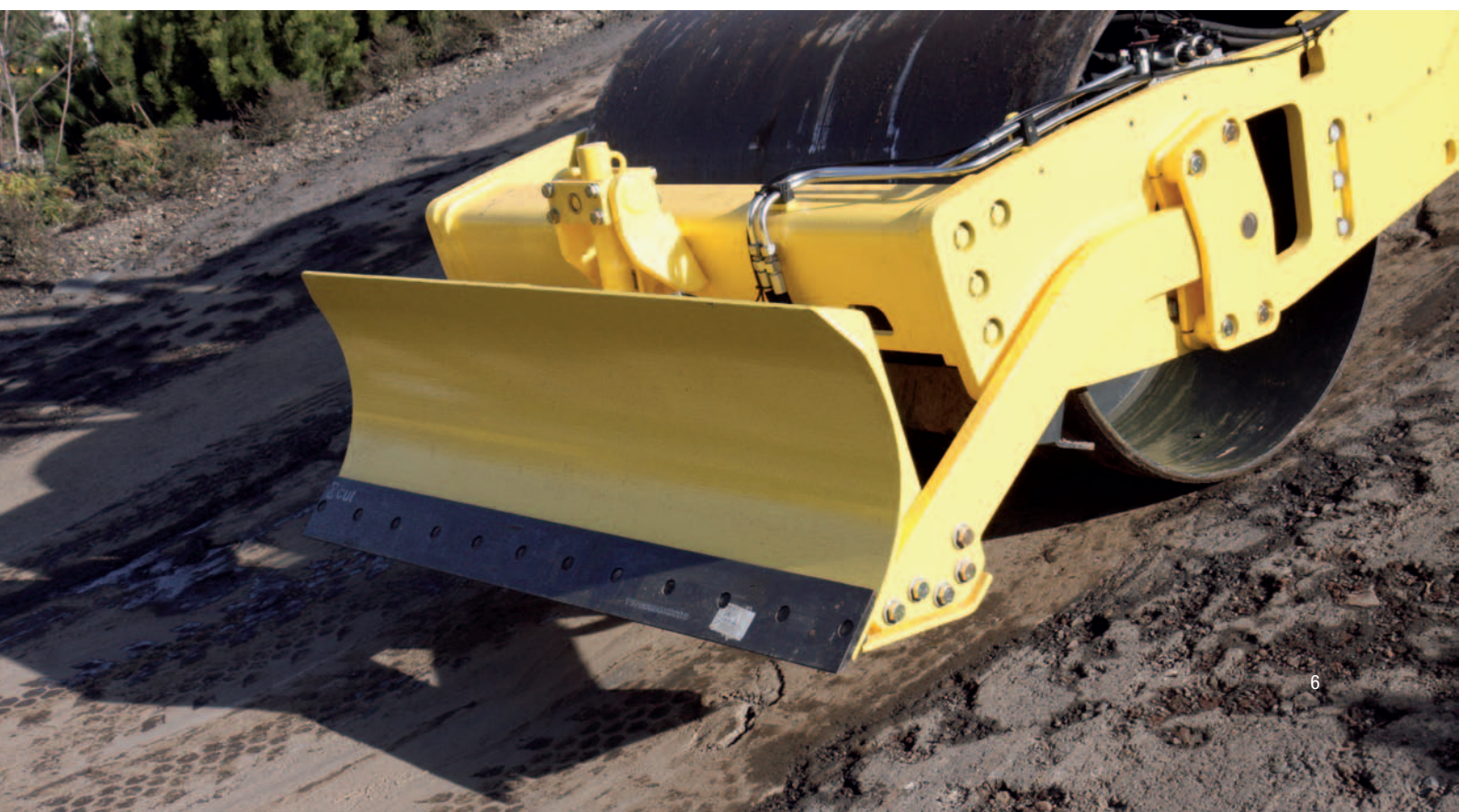
Dozer blade. Easy manual operation with the travel lever.
