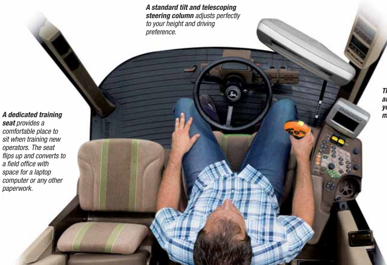
New GS2 overhead-mounted control panel puts access to GREENSTAR systems out of the way but within easy reach.
