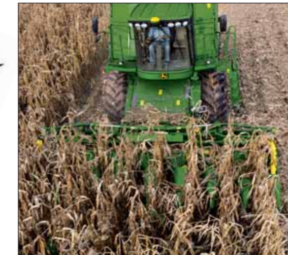
Optional CommandTouch Multi-Speed Feederhouse Drive System delivers higher capacity feeding in the heaviest yielding corn. A reliable PowrShift transmission provides up to 42% more torque capacity and enables operation of the cornhead in five speed ranges. Adjust the speed of your cornhead easily from the cab by pressing one button on the multi function lever and gain the advantages of more productivity and increased performance in corn harvest. And with the new larger feederhouse lift cylinders you are able to handle 12 row cornheads easily.
