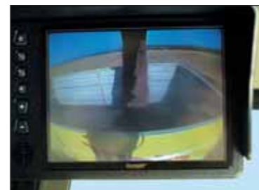
In-cab colour monitor and exterior cameras enable you to see behind the combine, as well as the unloading auger and trailer.
