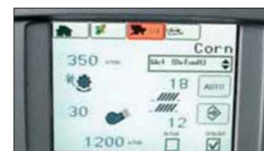
Automatic Combine Adjustment (ACA) gives you full, automatic adjustment of the rotor concave setting, cleaning fan and rotor speed, plus cleaning shoe settings.
