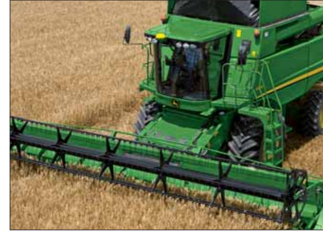
The feederhouse width perfectly matches the width of the threshing area, promoting smooth, uniform material flow and reducing the chance of slug feeding.
