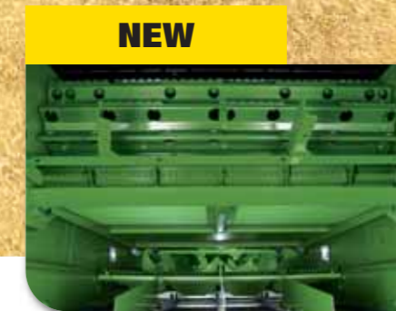
The new discharge beater housing design improves material flow to the chopper.
