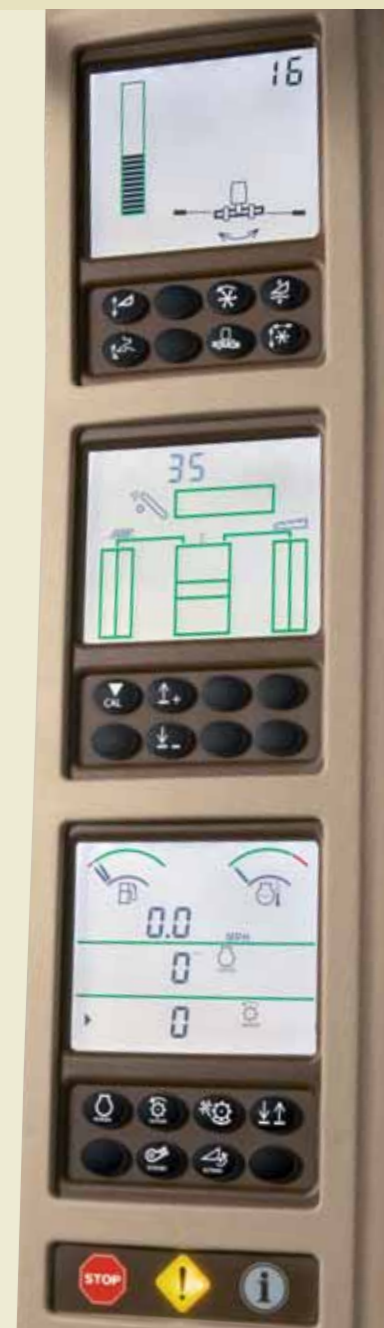
The triple display tachometer lets you monitor three functions simultaneously. In addition to ground speed (which is always shown on the top line) you can select engine rpm, cylinder rpm, concave clearance or cleaning fan speed. Anytime you touch or adjust any monitored combine function, it's automatically displayed on the bottom line.
