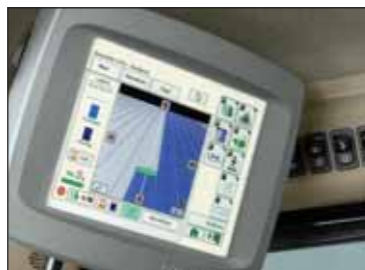
New GS2 overhead-mounted control panel puts access to GREENSTAR systems out of the way but within easy reach.
