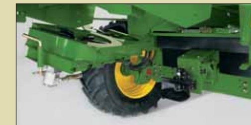
The chaff spreader is hinged for convenient access to the cleaning shoe.
