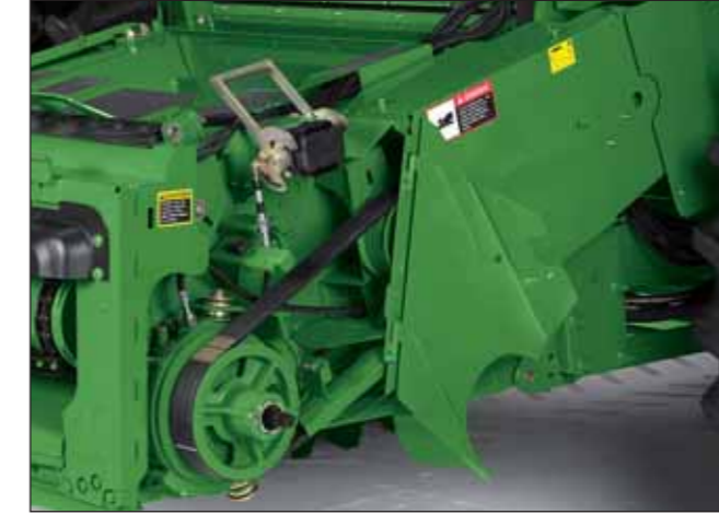
Reverse out blockages from the cab. The heavy duty reverser efficiently dislodges the worst platform and feederhouse blockages.
