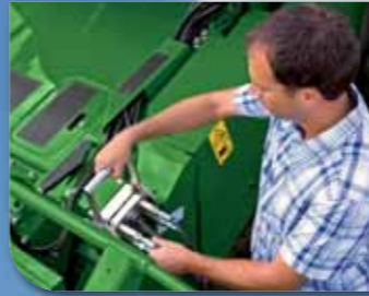
Single-lever latching gives you the ultimate in header hook-up convenience. One lever connects the electro-hydraulic multicoupler and engages the platform attachment pins. Fast, easy and clean.
