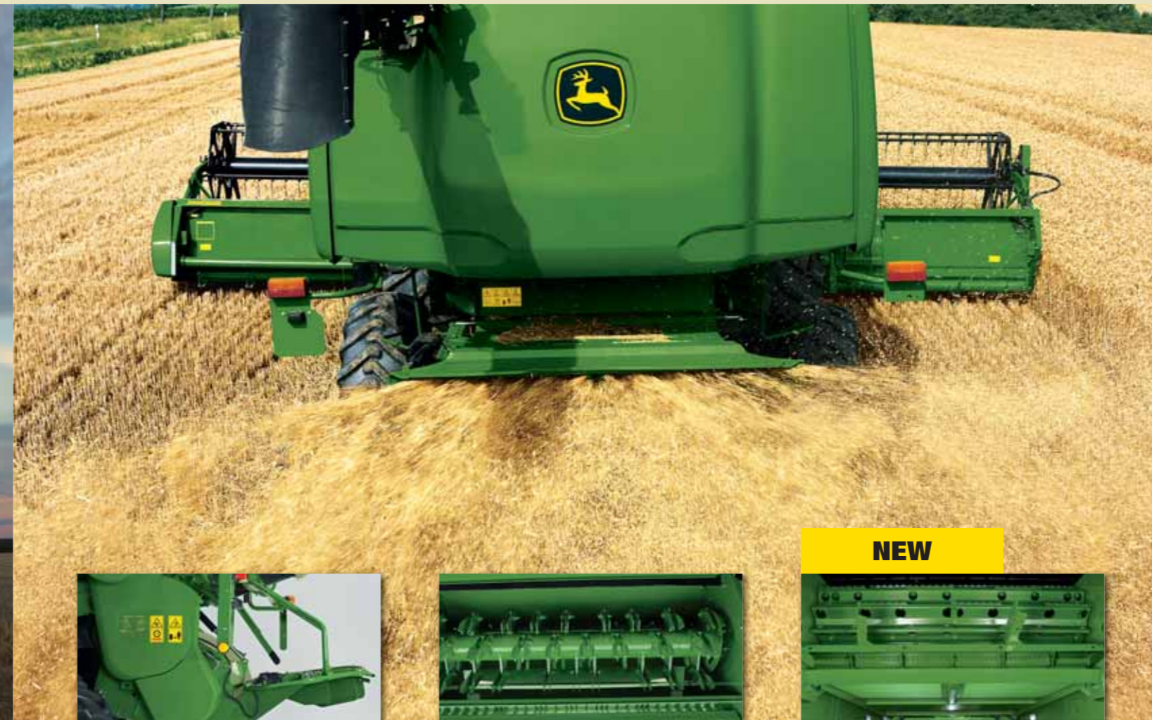
With the Premium Chopper* concept you are able to separate and spread the chaff when windrowing straw. Ideal for farmers who use the straw for baling and want an even spread of all cleaning shoe residue. Or direct the chaff into the flow of chopped straw for perfect distribution of the residue.
