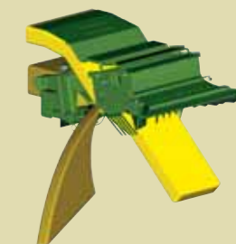
The chaff spreader discs change speed and direction of turning automatically when the chopper is moved between chopping and windrowing position. This ensures perfect distribution of chaff and straw up to the full cutting platform width in all crops and conditions.
