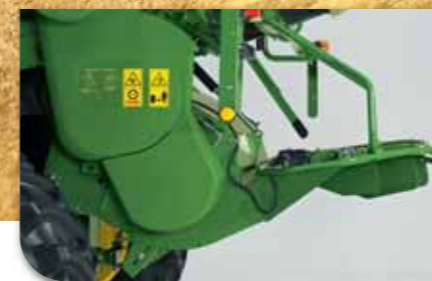
The extra fine cut chopper and spreader system chops and spreads residue from both the separator and cleaning shoe evenly over your field. Ideal for no till or minimum till applications.
