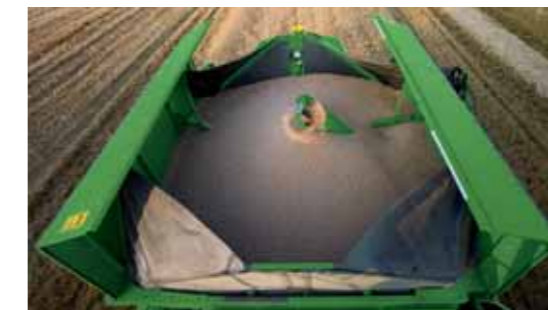
Grain tank covers open electrically from the operator's seat.
