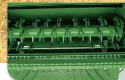
60 specially designed, low profile, serrated "Propeller Blade" knives accompany 60 straight serrated knives, which aggressively cut and distribute the straw and chaff evenly across the entire width of the platform. Choose either 1600 rpm for maize or 3200 rpm for small grain.
