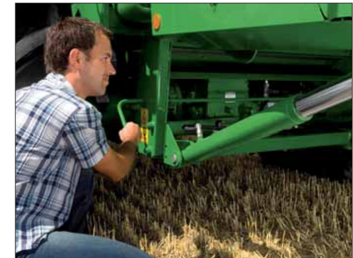
Now you can harvest close to the ground without worry , even in stony fields. The S690 stone trap catches stones before they reach the threshing module. Flip one lever for fast, easy cleaning.
