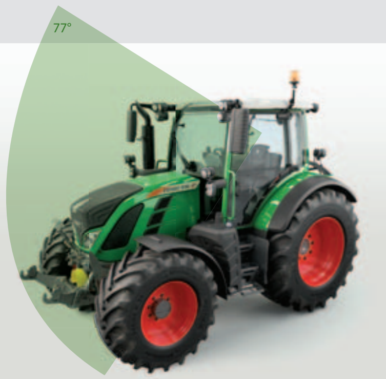
The upward viewing angle has been tripled. The downward sight lines have also been optimised and it is easy to see into the wheel arches.
