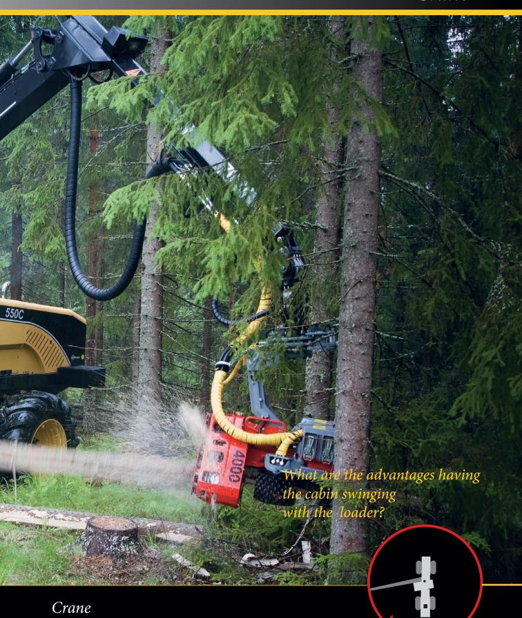
Lifting capacities from 180 kNm to 300 kNm. Also, depending on the models, different choices of reaches are available, from 9,5 m to 12,5 m. The crane functions are easily adjusted from the machine control system.
