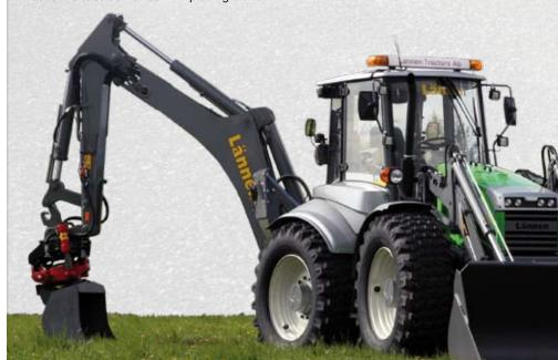
90 (123) kW (hp) 119 (162) kW (hp) 696 Nm
