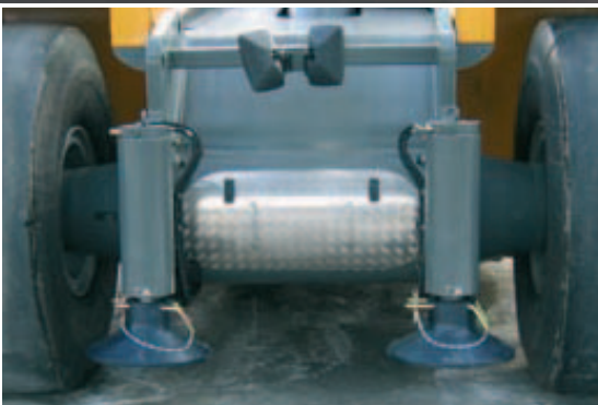
Supporting pads for increased lifting capacity in the second and third row (option).
