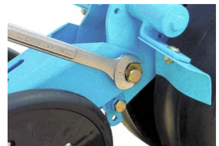
Turn the eccentric bolt to adjust the closing wheel bracket, allowing you to get an exact center on the unit.
