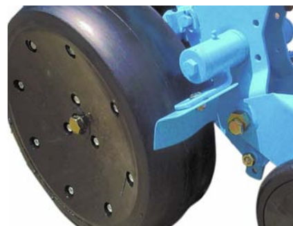
Scraper keeps the gauge wheels clean.
