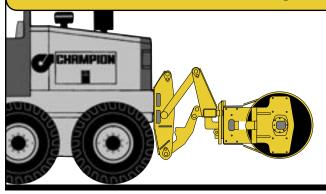
The Vibratory Compaction Roller is used for road maintenance applications. It can compact areas for road resurfacing and roll finished asphalt. This attachment eliminates the need for a separate compaction roller to be brought to the job.
