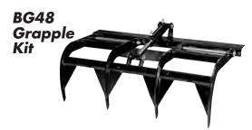
Mounts to DB480S, SB480TS, & SB480S Buckets (see page 4). Consists of four solid steel tines robotically welded to heavy-duty frame developing over 1,000 lbs of clamping force. Retracts completely to allow normal loader operations without removal. [Requires drilling (25) 3/8" holes in mating Bucket; Factory assembly available]
