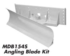
Mounts to Loader equipped with SH44 Speed Hitch. Uses Loader's hydraulics to control blade's lift. Adjust blade angle with single pin - no tools required. [Add CK29 Cylinder Kit (below left) for hydraulic angling] Blade is 54" wide, 17" high and 3/16" thick.
