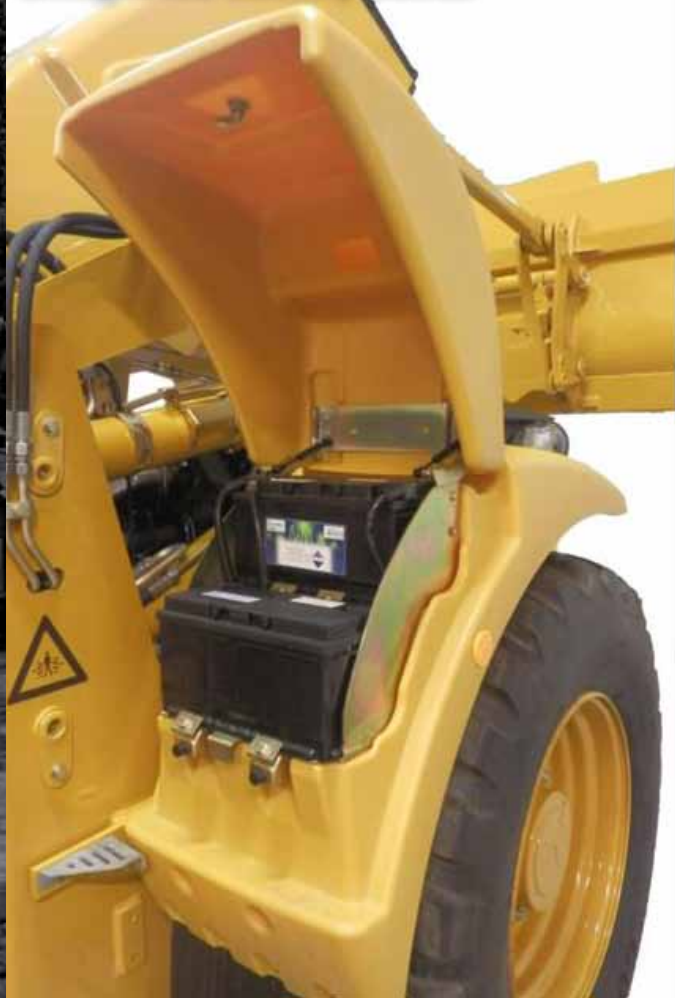
Integrated battery boxes
