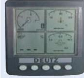
CAN bus display for the separate engine
