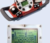
The clear display on the remote control provides up-to-date feedback and system information about the machine. Various parameters can be set here. The strength of the radio signal and charge status of the battery is indicated via bars.
