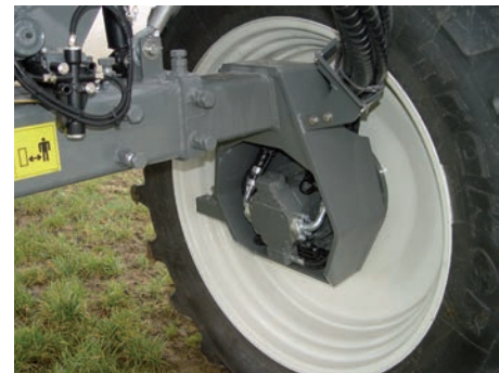
Hydrostatic transmission - 40 km/h
