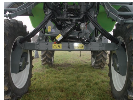
Mechanical and hydraulic track width adjustment (option)
